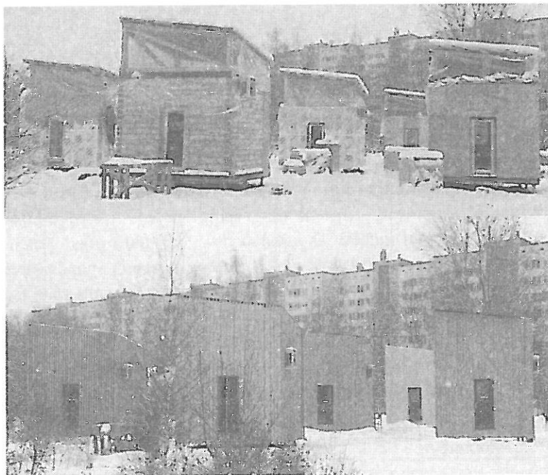
Fig 1. Polygon of test stands. Above: in the front – test stand of wooden logs; to the left – test stand of aerated concrete; at the back – test stand of plywood panels. Below: the completed test stands.
