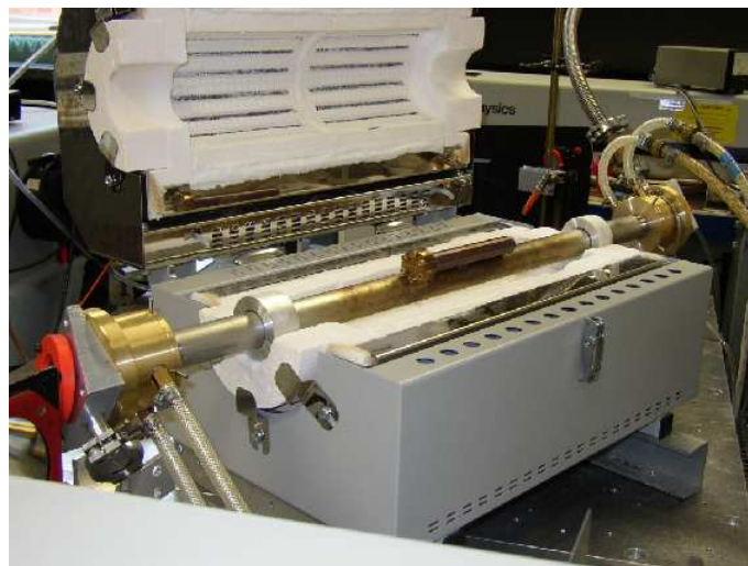
Figure 3.5. Oven with the NaCs heat-pipe.
