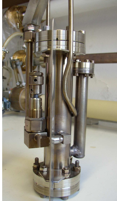
Figure 3.4. Metal cell used for experiments with NaCs.
