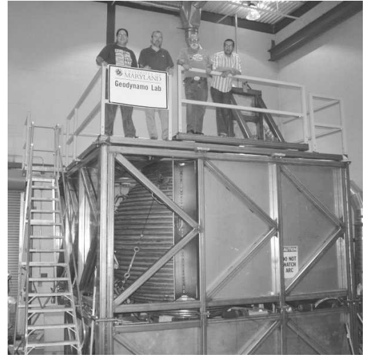
Fig. 20 The rotating 3m sphere in Maryland. An impressive video is available under www.youtube.com . Figure courtesy of D. Lathrop.
