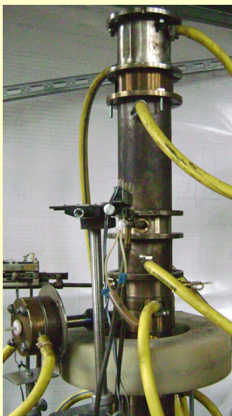
Magnetically controlled combustion apparatus in the laboratories of IPUL Credits : M. Zake
