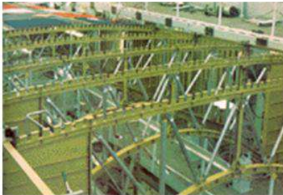
Figure 1. Mid-fuselage structure of Space Shuttle Orbiter showing boron-aluminum tubes. (Photo courtesy of U.S. Air Force/NASA ).
