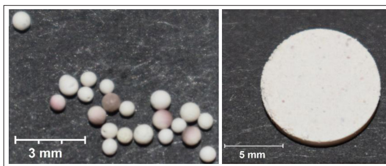
Fig. 1. The modified \text{Li}_4\text{SiO}_4 pebbles with additions of \text{TiO}_2 (Sample #1) – left, and pressed pellet – right
