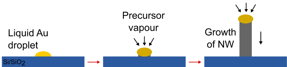
Figure 3.1. A schematic representation of vapour-liquid-solid growth mechanism.
