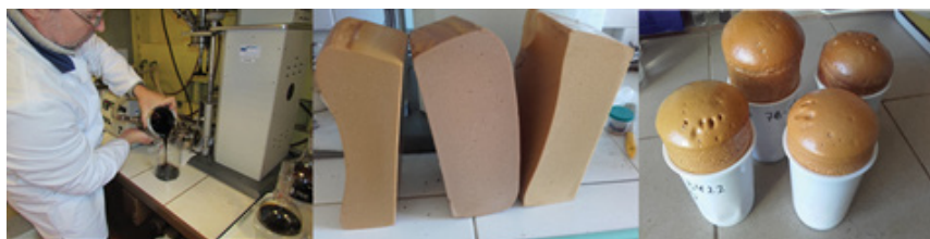
Figure 8. Lignopolyurethane foams derived on the basis of oxypropylated wheat straw lignin
