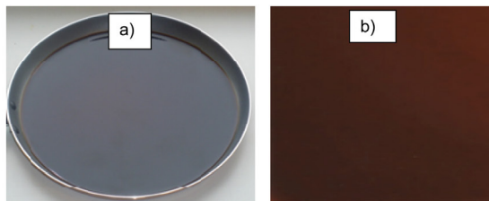
Fig. 1. LPU film, containing 20% of MET-F: a) under curing in a mold; b) cured and eliminated sample.
