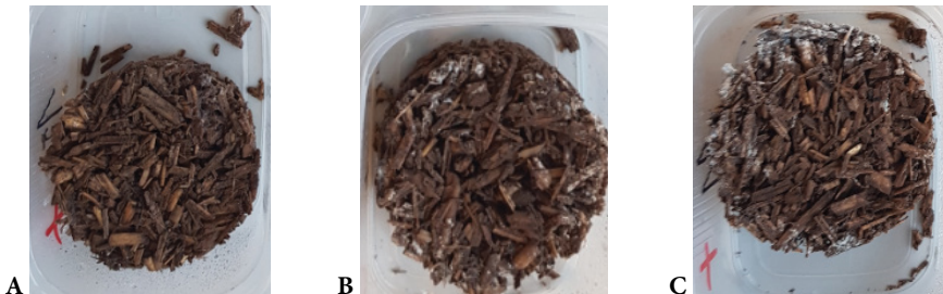
Fig. 3.11. Magnesium phosphate biocomposites with varying binder amount: A) MPC-100; B) MPC-50; C) MPC-20.
