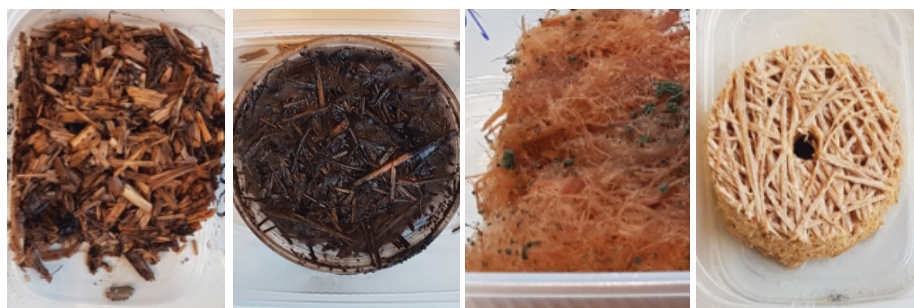
Figure 3.8. Materials after microbiological stability tests A) hemp shives; B) flax shives, C) wood wool; D) wood fibre cement board
