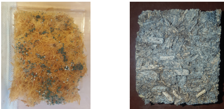
Figure 3.6. Control samples of wood wool covered with Trichoderma (A) and MPC composite covered with Penicillium and Aspergillus (B).
