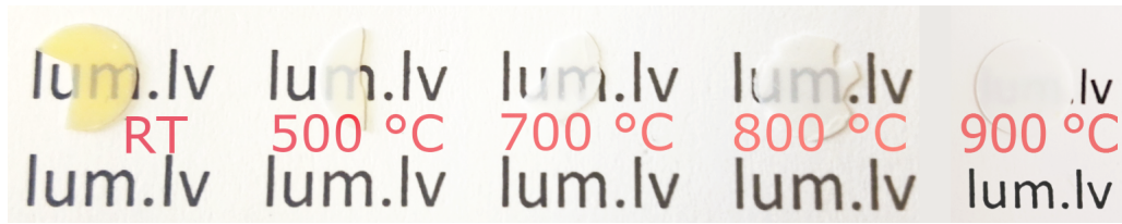
Figure 4.9: Pressed pellet with no annealing (RT) and annealing at 500°C, 700°C, 800°C and 900°C temperatures (right).
