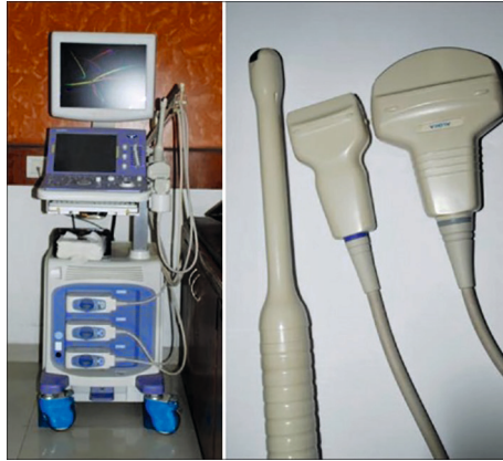
Figure 16. (On the left) High-frequency ultrasound machine with 7.5–15 MHz multi frequency probe with color and pulsed Doppler ultrasonography. And untrasound probes (on the right) [57]
