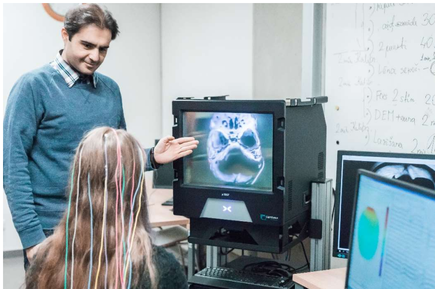
Figure 18. The volumetric multiplanar display employed for the 3D image presentation.
