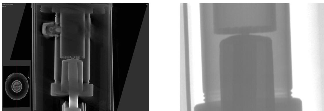
(a) CT image of failed ion source
