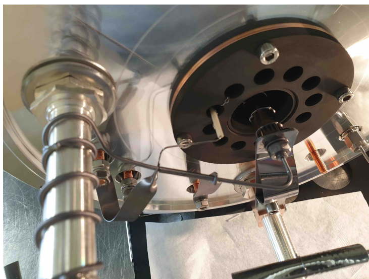
Figure 5.12: Assembly of the TISS #731 oven and gas line.
